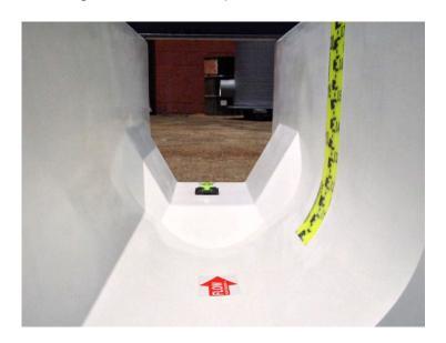
When using a staff gauge on a non-vertical surface it is important to know if the reading is corrected or uncorrected. For non-vertical applications, Openchannelflow indicates the primary device that the gauge has been designed (calibrated) for.
