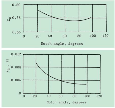
Note that the equation and correction factors apply to fully contracted V-notches. Partially contracted  $(90^{\circ})$ V-notches rely on different  $C_{a}$  values.
